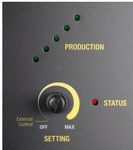
Once the salt level in the pool is correct the unit may be switched ON. The OPERATION LED will be green, and no cell output will be seen for approx. 120 seconds, this allows the pump and filter to prime and the cell housing to fill with water. After this start-up delay, the bar meter should light up showing all five LEDs. At this point the OPERATION LED should be green; if it is red it indicates that there is a problem and please refer to the table below.
