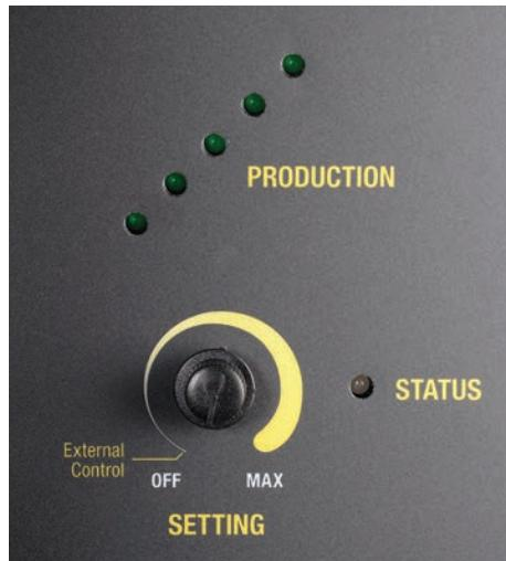
The external control input requires normally open (NO), voltage free contacts, where open contacts signal the chlorinator output is OFF and closed contacts signal the chlorinator output is ON. The external controller's output is connected to the terminals located at the base of the chlorinator as shown on page 6.
