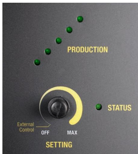
The unit is fitted with an electronic control and warning system. This regulates the output of the Unit to a preset maximum. The warning system consists of an OPERATION LED which will glow Red to indicate possible faults with the Unit or damaging operating conditions.
