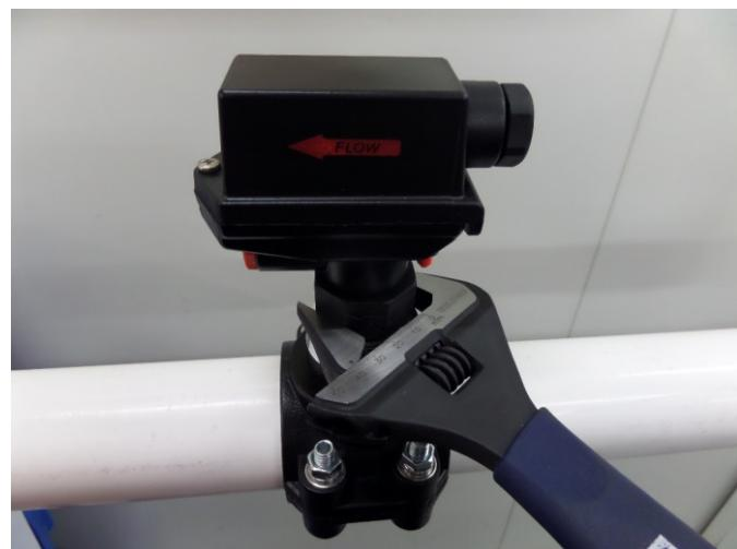
Alignment of the switch is critical to correct operation. The switch should be in line with the pipe and the flow arrow in the direction of flow. Remove the lid on the electrical enclosure and insert the wires into the cable entry. Connect the wires to the terminals labelled "COMM" and "NO".
