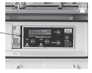
Pressing and holding "P1" will activate Pump 1 output and then Relay 1 in a continuous sequence. .
