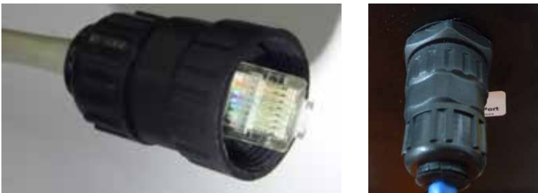
Figure 7.1: RJ45 Plug installed in housing (from rear)
