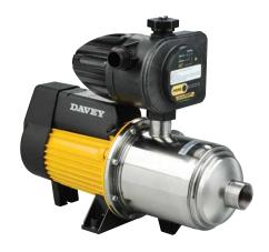
Torrium2 controlled HM Series provides a constant flow water supply system with an all stainless steel pump unit. The Torrium2 is adaptive, eliminating cycling, provides loss of prime protection and over temperature cut out. Pressure tanks can be added if site conditions require additional draw off.
